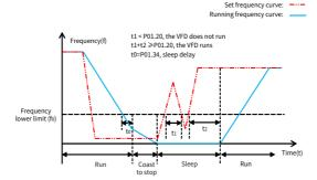
When the set frequency is lower than the frequency lower limit, and the ones place of P01.19 is set to sleep, the VFD stops according to the tens place of P01.19 and sleeps once running at the lower limit for the time specified by P01.34. If the set frequency is higher than the lower limit once again and it lasts for the time specified by P01.20, the VFD restores to the running state automatically and increases to the set frequency.
