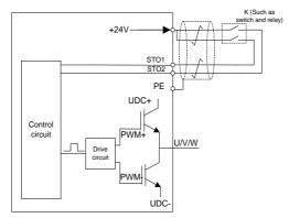
Figure F-2 STO function circuit internal power wiring
