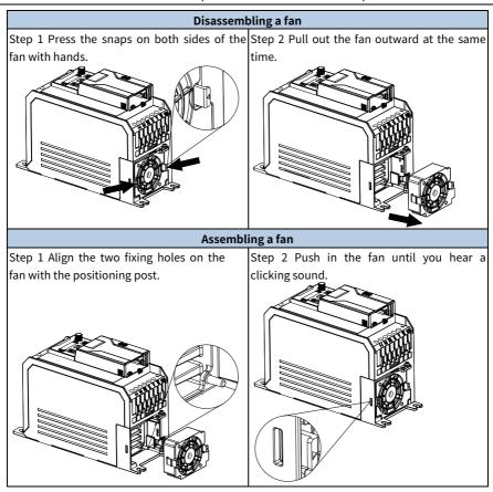
**Note:** Before disassembling or installing the VFD, stop the VFD, cut off the power, and wait at least 5 minutes.
