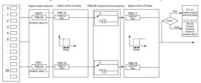
The following table lists the options of function parameters P06.04–P06.05. A same output terminal function can be repeatedly selected.
