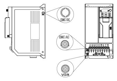
Figure 4-3 EMC screw positions (for frames D and E)
