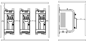
**∠Note:** The ambient temperature for side-by-side installation must not exceed 40°C.
