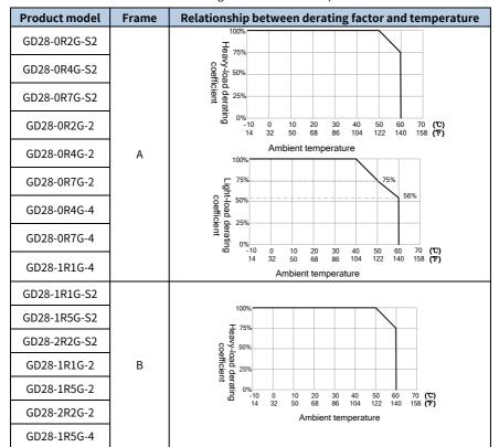
Table B-1 Derating due to ambient temperature
