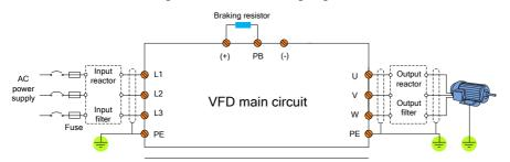
**∠Note:** The fuse, input reactor, input filter, output reactor, and output filter are optional parts. For details, see Appendix E Peripheral accessories.
