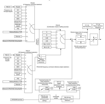
When P05.01 or P05.02 is 10 or 11, DI1 or DI2 is the UP or DOWN terminal. When DI1 or DI2 is closed, the reference frequency will be fast increased or decreased. The increase or decrease rate is determined by P08.47 or P08.48. See the following figure.
