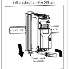
snap slot and rotate it 90 degrees to release the snap on that side. Repeat the same method to remove the snap on the other side.
