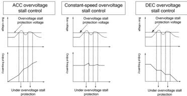
Figure 6-1 Actions taken for protection against overvoltage stall
