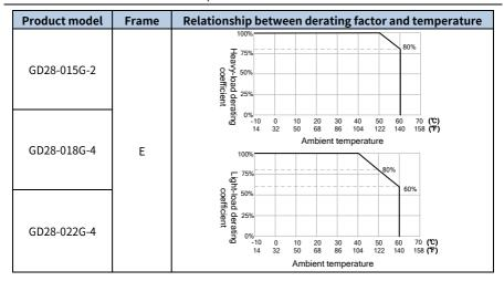
**✓Note:** It is not recommended to use the VFD at an environment with the temperature higher than 60°C. If you do, you shall be held accountable for the consequences caused.
