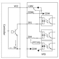
NPN (sinking) mode (Internal + 24V power supply)
