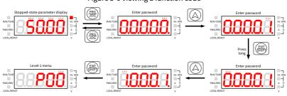
Figure 5-6 Viewing a function code
