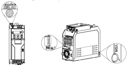
Figure 4-2 EMC screw positions (for frame C)
