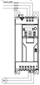
Figure 4-23 Fuse configuration
